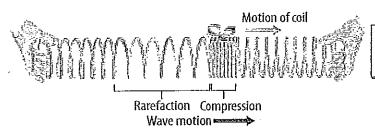
The wave makes the coil with the yarn move to the right as the compression of the wave reaches that coil.
